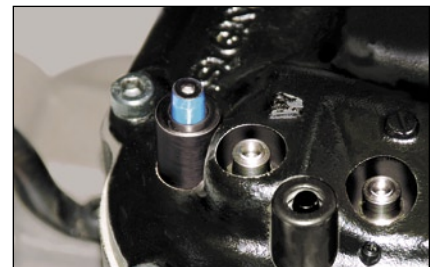
Minimum air pressure indicator button appears "blue" to confirm that minimum air pressure is available for tool operation.
